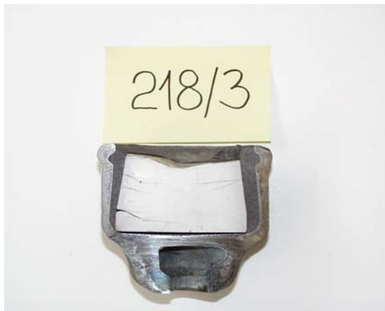
Figure 5. Transverse cuts and network of thin cracks in the head of the broken insulator
